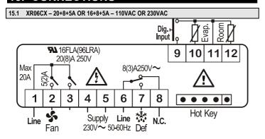
NOTE: The compressor relay is 20(8)A or 16(6)A depending on the model.
