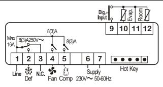
NOTE: Connect the 120Vac power supply to 6-7
